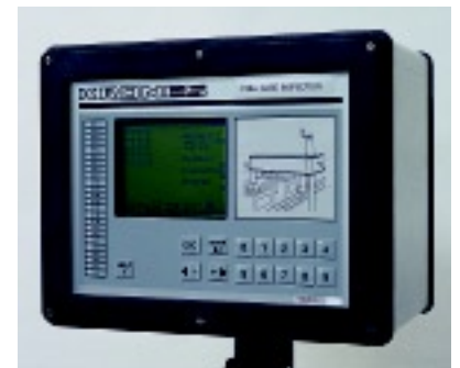
Full carton inspection with the Checkmat VK-W with weighing unit (above)
