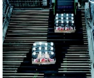
Sorting of non-conforming trays via transversal distribution unit
